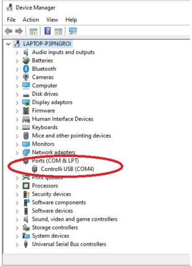
Figure 18. Windows device manager to identify the COM port of the actuator
